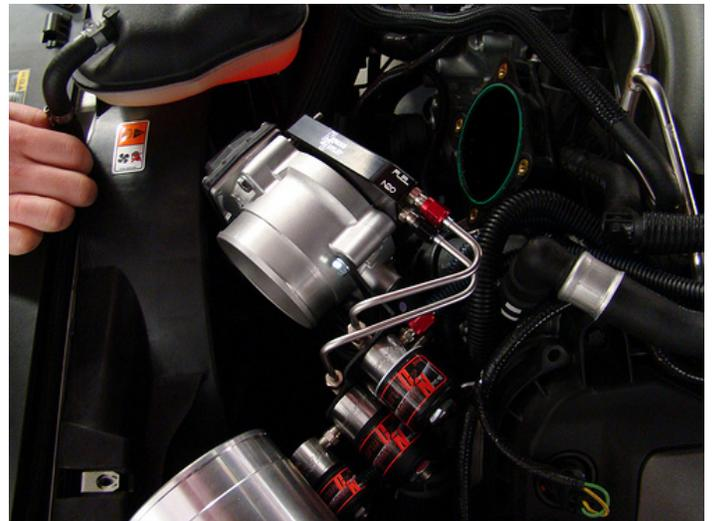
**Step 5** Remove the (4) 10MM stock mounting bolts from the throttle body, as you remove the throttle body, flip it to unplug the motor plug on the bottom. This is done by pulling the red tab back and pulling the connector away from the connection point.
