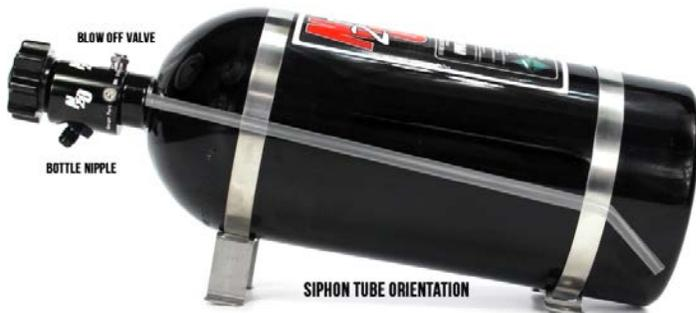
Bottle placement is critical to the performance of your nitrous system. It is important to mount your nitrous bottle properly in order to ensure that the siphon tube located in the nitrous bottle picks up liquid nitrous.
