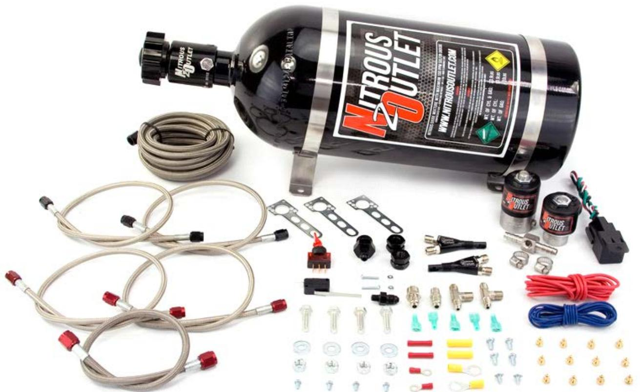
Your system should come with everything you see here, the fuel feed/adaptor fitting may vary for vehicle specific systems. You will have everything you need to install a nitrous system on your vehicle; main feed line, fuel adapter fitting, nitrous and fuel lines, solenoids and brackets, electrical fittings and wire, relay and harness, bottle brackets, wide open throttle switch, toggle switch for system arm, nozzle and nozzle adapter, jetting for up to 200HP.
